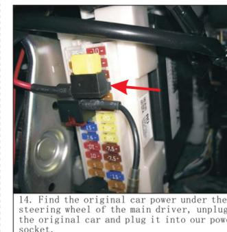
14. Find the original car power under the steering wheel of the main driver, unplug the original car and plug it into our power socket.
