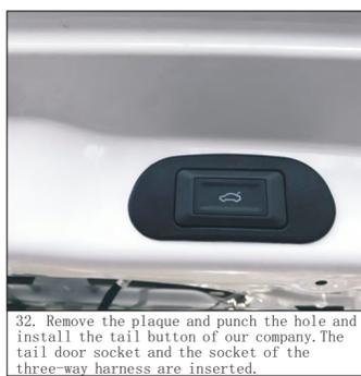
32. Remove the plaque and punch the hole and install the tail button of our company. The tail door socket and the socket of the three-way harness are inserted.
