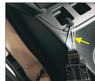
12. The front switch ILL cable is connected to the white green cable of the original car small lamp terminal housing.
