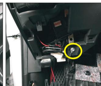
13. The front switch ground wire is connected to the grounding screw below the main steering wheel.
