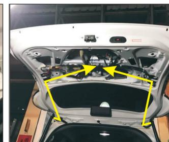
8. Strut cable runs along the yellow cable to the tailgate cover
