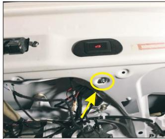
31. Control box installation position, fixed with our screws, gaskets and mesons
