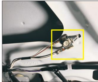
19. Locate the grounding screw at the tailgate. Connect the screw to our power ground.
