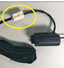
25. As shown in the figure, the socket of the electric suction lock is inserted into our electric suction Hall line socket.
