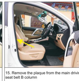
15. Remove the plaque from the main driving seat belt B column
