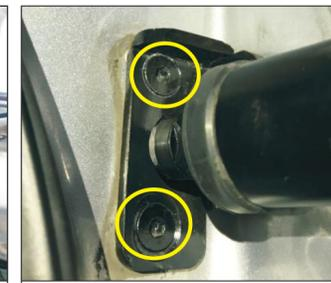
3. Remove the lower right bracket of the car, install the lower right bracket of our company, and fix the bracket with our screws
