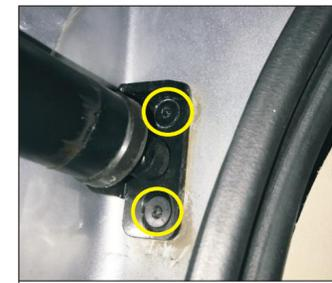
4. Remove the left lower bracket of the original car, install the left lower bracket of our company, and fix it with our screws
