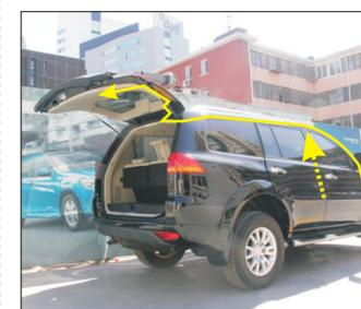
20. The main driving power wire, the front switching wire and the center control wire are routed from the top of the vehicle along the yellow arrow to the tailgate cover
