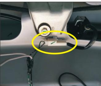
20. Find this terminal housing at the back door and insert the front switch adapter
