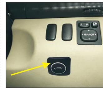
12. The main driver removes the cover on the right side of the steering wheel, punches and installs the front switch button of our company.
