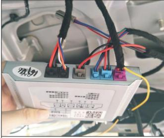
28. The control box plug is plugged by the color, check the plug in place, and finally insert the purple power cord socket
