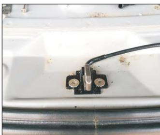
24. Remove the original car lock, install our electric suction lock, use our screws to fix
