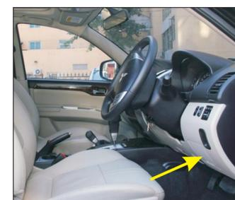
18. The power wire, the front switch wire, and the center wire are routed from the top of the vehicle along the yellow arrow to the tailgate cover
