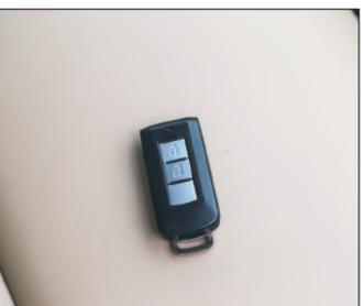
Press the remote control unlock button for 3 seconds to open/close the tailgate
