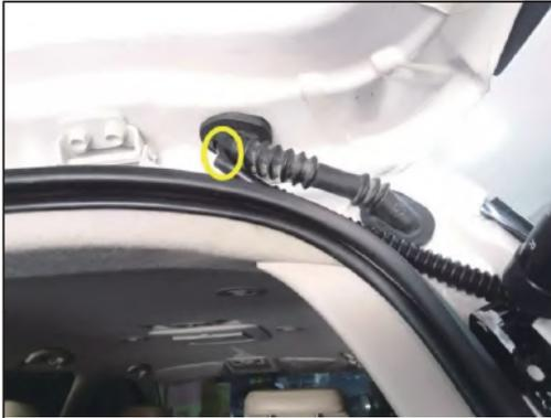
5.Punch holes in the waterproof plug and the Hall line passes through the holes.
