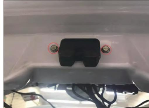
18.Install our electric suction lock and fix it with original screw
