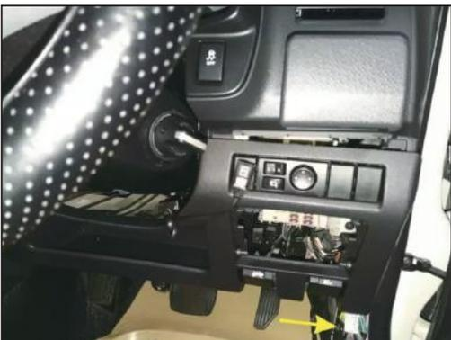
10.Remove the trim at the lower right of the power supply and find the ground wire
