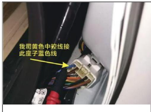
12.Remove the trim board at the B pillar of the right main driver's seat belt and find the original car central control. Our company's central control wire connects the blue line of the seat.
