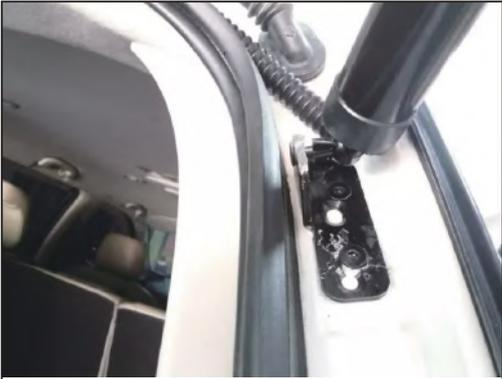
4.Remove the right lower bracket of the original car, install the right lower bracket of our company and fix it with our company's screw
