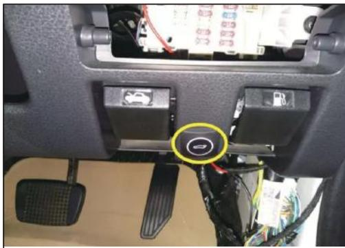
13.Punch holes in the lower panel of the power supply and install the front switch of our company
