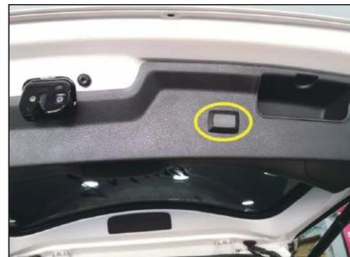
21.Punch holes in the tail door panel, install the tail door button of our company, and restore the panel.
