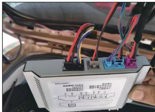
20.Plug Hall wire, power cord and electric suction wire into control box one by one according to color
