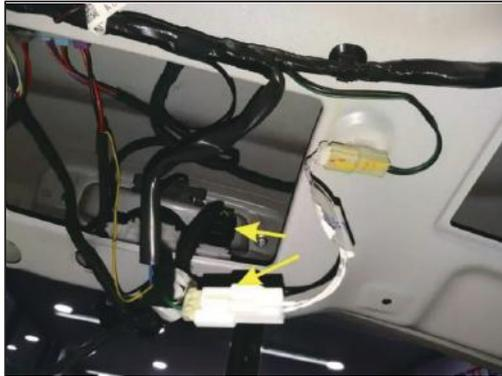
16.Pull out the plug at the rear door lock and plug in the three-way socket of our company. The other end plug of our company's three-way socket is plugged in the original door lock.
