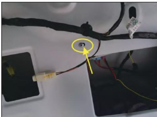
19.Install our central control box and fix it with our screw and gasket
