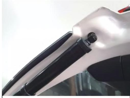
3.Install our support rod with the ball head of the original car (the same steps are left and right)
