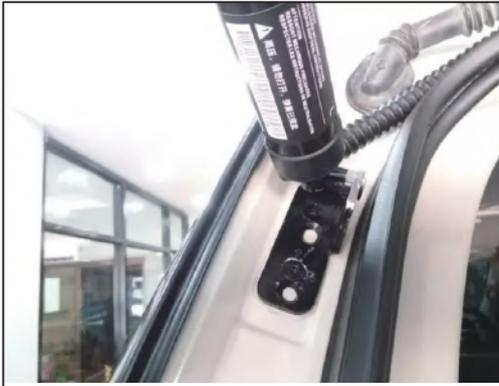
2.Remove the left lower bracket and support rod of the original vehicle, install the left lower bracket of our company, and fix it with our company's screw. Note: Someone needs to hold the door.
