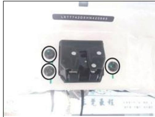
12. Remove the door lock of the original vehicle, install our electric suction lock, and fix it with the screws of the original vehicle.
