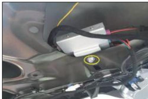
14. Installation position of control box, fixed with our screw, ring and flat washer
