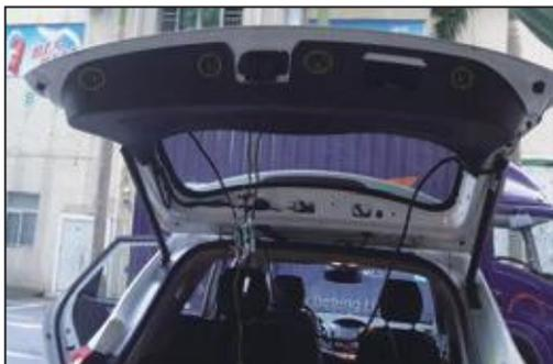
1. Remove the button and remove the trim panel
