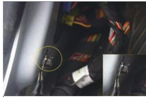
9. Main driver compartment side connection to ground wire
