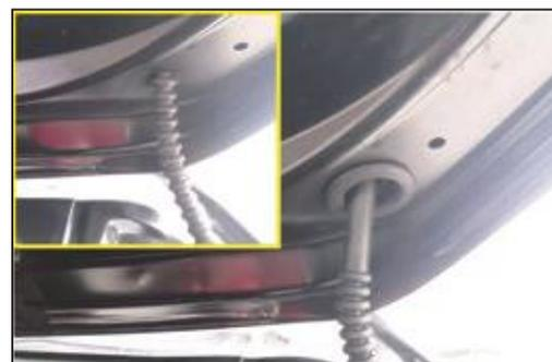
6. As shown in the figure, the hall line passes through the reserved hole and plug in the rubber plug (the same as the left and right steps).
