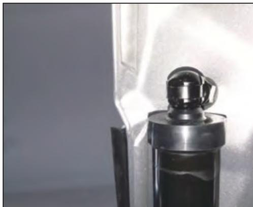
2. Remove the ball head of the original vehicle and install the specially designed electric pole with the specially designed ball head.
