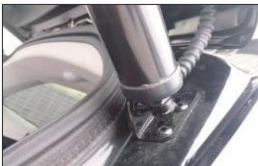
4. Remove the right lower bracket of the original vehicle, install the specially designed lower right bracket, and fix it with the specially designed round head screw (as shown in the figure).
