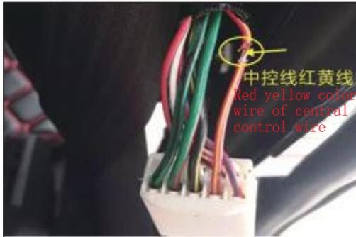
10. Remove the trim board at the B-pillar of the main driver's seat belt and find the central control. Our yellow central control wire connects the red and yellow line of the seat (the fourth hole in the first row from left to right).
