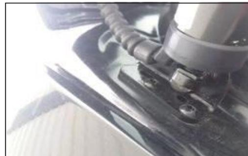
3. Remove the left lower bracket of the original vehicle, install the special left lower bracket, and fix it with the specially designed round head screw.
