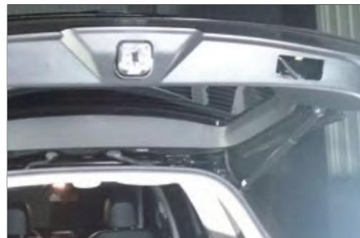
15. Remove the trim board, punch holes in the trim board and install the tailgate switch button.
