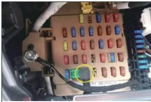
8. Remove the trim board under the main driver, pull out the 15A fuse of the original car and insert our power plug into it.
