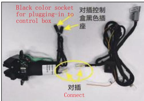
13. As shown in the figure, connect our electric suction lock socket.
